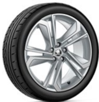
Libra light-alloy wheel 7J x 18" ET51 for 215/40 R18 tyre
