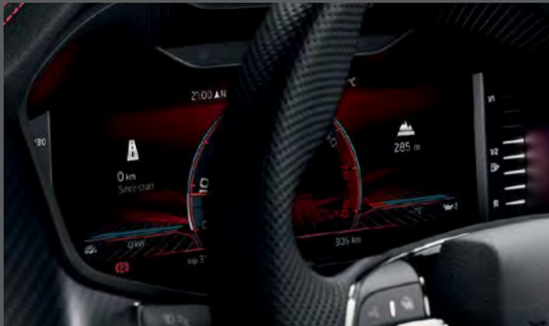
VIRTUAL COCKPIT The 10.25" digital display replaces the traditional instrument display and can be customised with five views (Classic, Basic, Extended, Modern and Sports).
