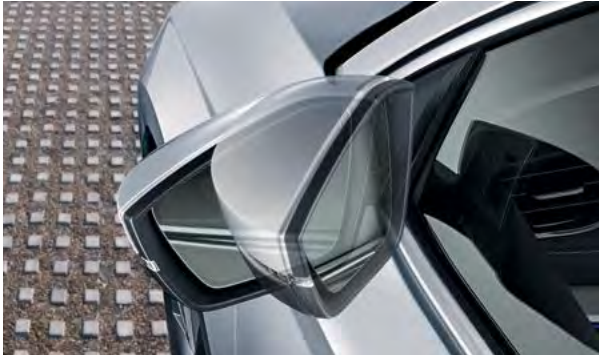
ELECTRICALLY ADJUSTABLE, HEATED, FOLDING AND DRIVER SIDE AUTO-DIMMING DOOR MIRRORS
