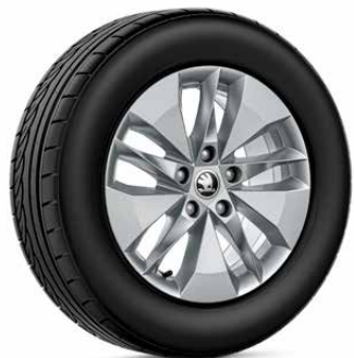
Twister light-alloy wheel 7.0J x 16" ET46 for 205/60 R16 tyres
