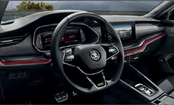
SPORT STEERING WHEEL The OCTAVIA vRS is equipped with a three-spoke leather sports multi-function steering wheel with paddles for DSG.
