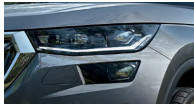
Full LED Matrix headlights with AFS (adaptive front light system), cornering function and AWL (all weather lighting system)
