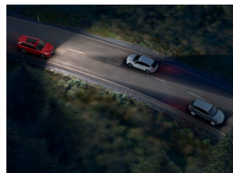
Full LED Matrix headlights with AFS (adaptive front light system), cornering function and AWL (all weather lighting system)
